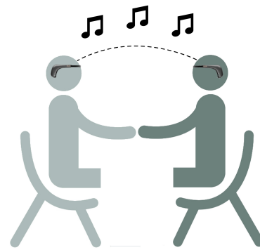
Figure 1: The basic use context of our auditory instrument. Two people (a “dyad”) engage with each other in face-to-face communication while networked Muse EEG headsets transform transient inter-brain similarity into music.
